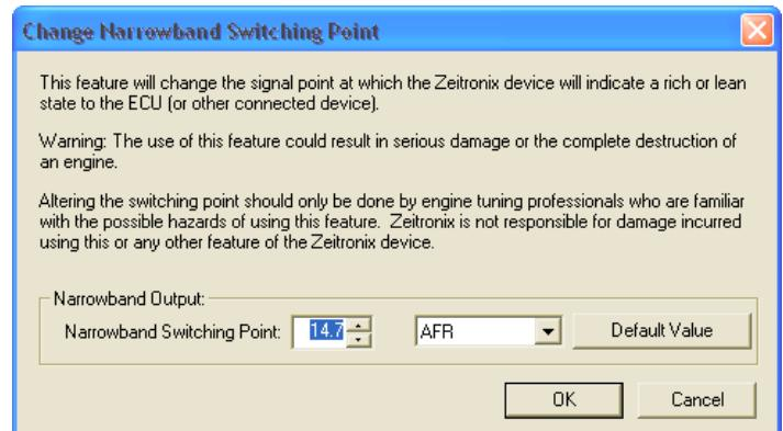
To Change the Narrowband Switching Point, adjust the number in the menu and click OK. The Narrowband Switching Point can be restored to a default value of 14.7 AFR by clicking on the Default Value, then OK.
