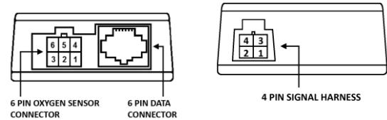
WHITE and BLACK wires can be used to provide a linear wideband signal and ground to a 3<sup>rd</sup> party engine management system. Data port is used to interface digitally with Zeitronix gauges, displays and third party loggers. For true plug and play, Zeitronix gauges and displays are powered directly from the Zt-3 Data port.
